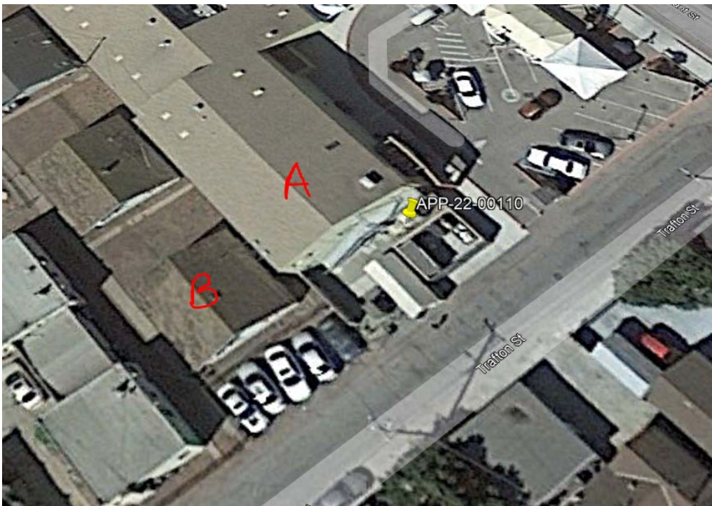
Figure 2. Adjacent buildings included in building downwash on AERMOD.
